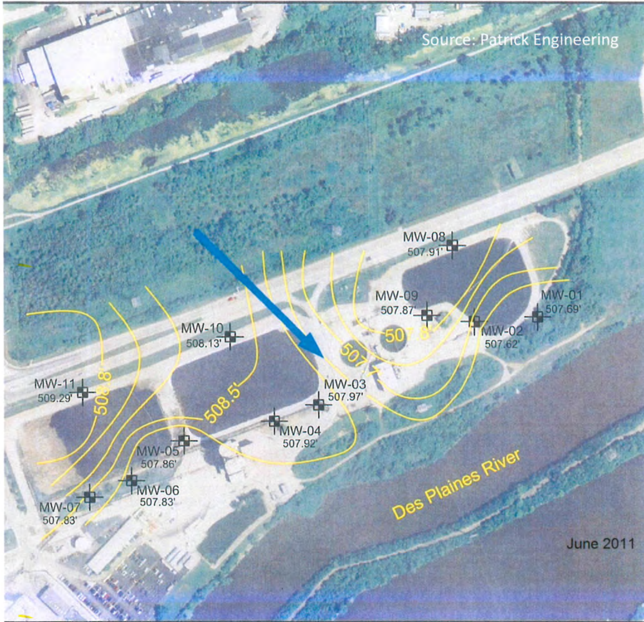
Figure 3 June 2011 Second Quarter Ground-water Contours Showing Mounding Beneath the Joliet Ash Ponds (PCB 2013-015)
